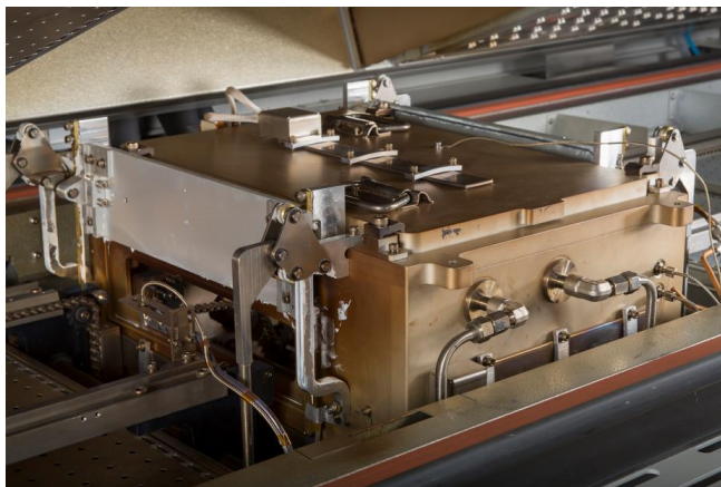
Figure 6. Vacuum reflow chamber shown within the convection reflow oven.
